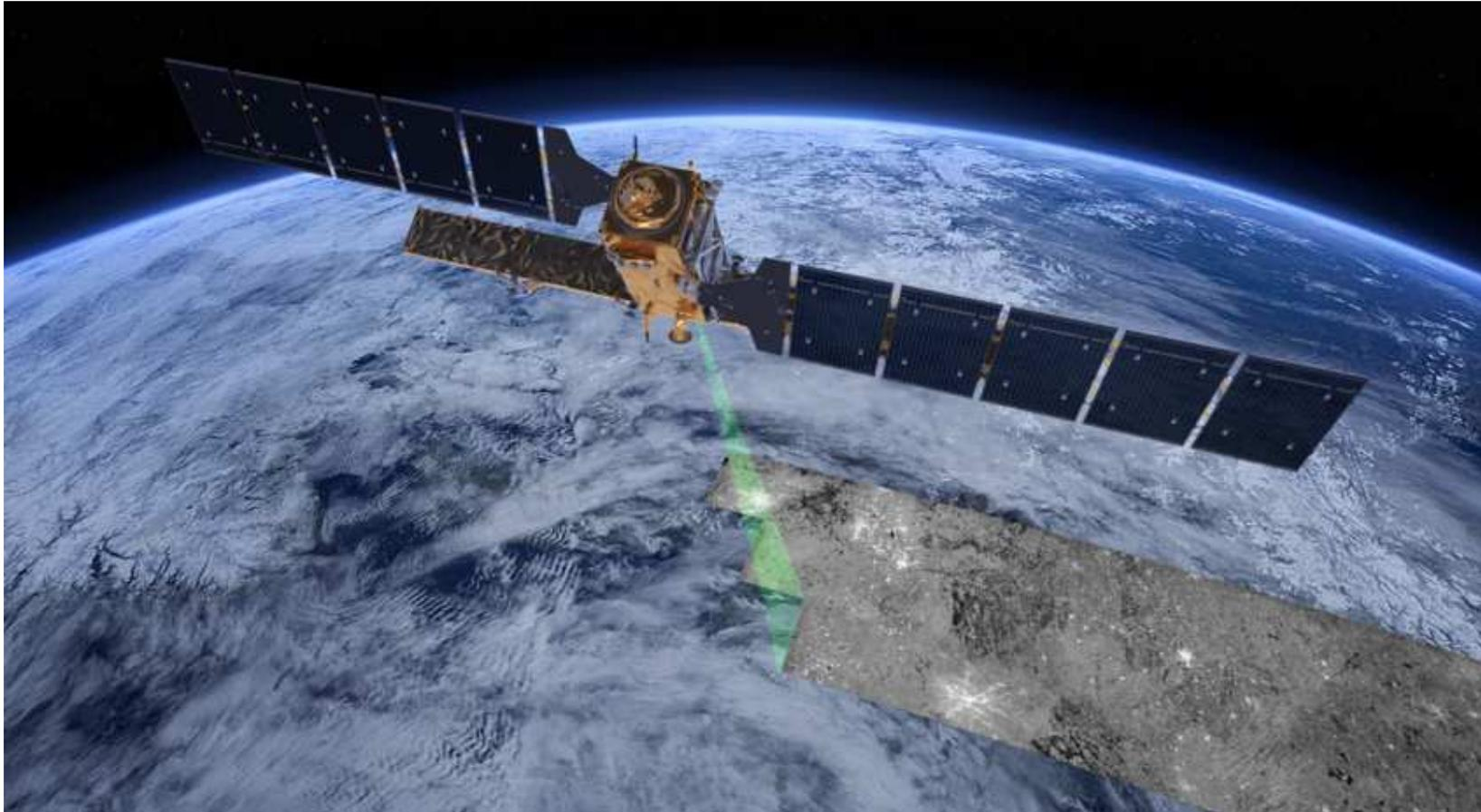
*“Sentinel-1 is a constellation of **two satellites** operating **C-Band Synthetic Aperture Radar imaging** with resolution down to 5 meters. The two satellites offer a six-day exact repeat cycle and their data are delivered to service segment within an hour of acquisition. Sentinel-1 is applied in several fields, such as agriculture oceanography, geophysical monitoring of natural hazards, time-series analysis of surface deformation, digital elevation mapping, etc.” (ESA, 2013).*
